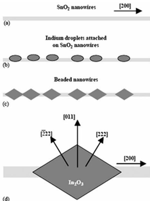
Fig. 4. The formation process and structural models of the beaded nanowires. (a) First,  $\text{SnO}_2$  nanowires form. (b) In droplets attach on  $\text{SnO}_2$  nanowires. (c) Beaded nanowires form. (d) Schematic diagram of the structural relationships of the faceted beaded nanowires [17]
