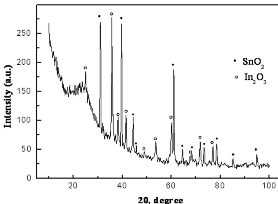
Fig. 2. XRD pattern of the beaded nanowires. The rutile-structured  $\text{SnO}_2$  and cubic-structured  $\text{In}_2\text{O}_3$  can be indexed
